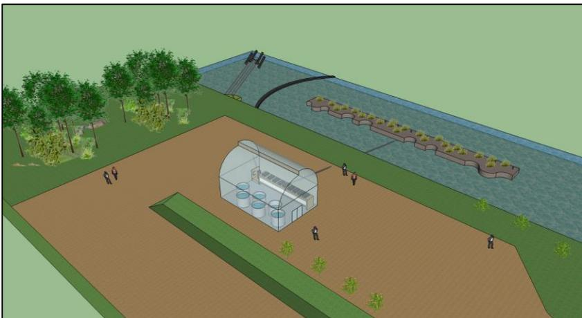
*The system consists of four interlinking technologies: a greenhouse with solar aquatic tanks and a mycelial loop, a floating plant raft anchored in the canal and a sediment intake structure.*
